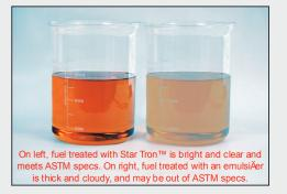
generally associated with oil/water emulsions will thicken the fuel. Thickened fuel can destroy a fuel pump and fuel injectors. The ASTM specifications for fuel viscosity are very concise; thickening the fuel with water can take the fuel outside its specifications, which can void a warranty.
